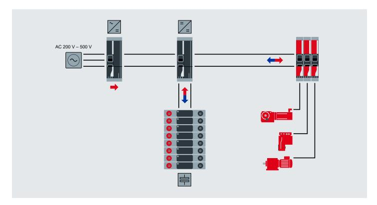
Software modules facilitate the automatic synchronization and switching on of the storage unit and the variable control on the DC link side or energy storage unit side with dynamically adjustable power limiting and current limiting.
