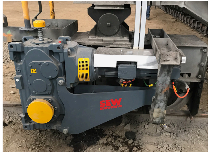
After: A more enclosed, high-efficiency drop-in replacement offers better protection from harsh elements.
