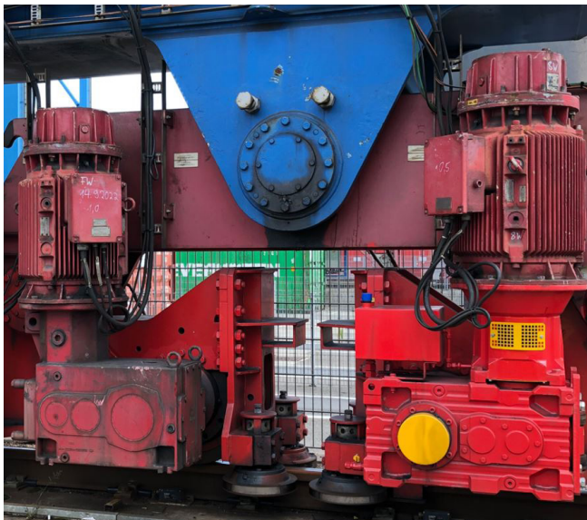
A new gearbox (right) is simply dropped into an existing system with minimal downtime.
