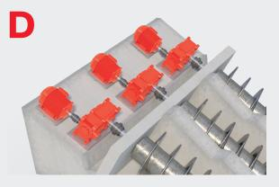
Motor and helical gear unit are connected by an elastic claw coupling.
