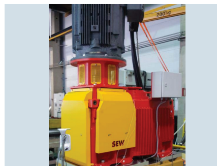
Flotation cell drive
