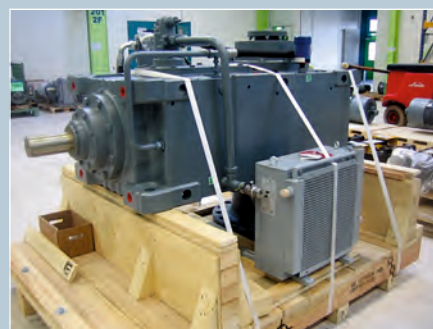
Flotation cell drive
