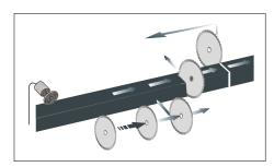
In the case of flying saws, MOVIKIT® MultiMotion Gearing is used for synchronous operation between several axes. The interpolation add-on is used for customized travel profiles, while the CombinedEncoderInterface add-on is used for combined encoder evaluation.
