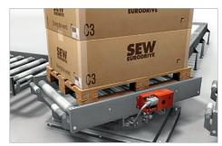
Materials handling technology with changes of direction Rotary table, carriage
