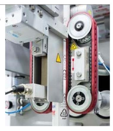
This FFS machine packages a product in film. To ensure error-free packaging, a sensor detects the print marks on the film and passes on this position information to the controller so that any necessary corrections can be made.
