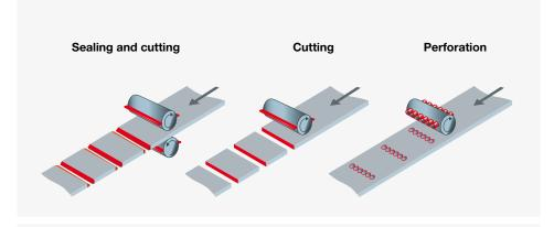
In this example, two rotary knives are A rotary knife cuts material into used for sealing and cutting in a horizontal form, fill, and seal machine.
