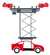
MOVIKIT® MultiAxisController Torque eliminates any torque stresses between the two drives in this electrified monorail system.
