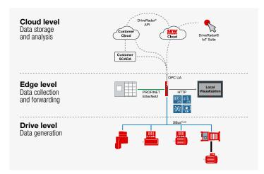
MOVIKIT® DeviceIdentity and MOVIKIT® DeviceVitality are used as software-based smart services at edge level to create the connection between automation and IoT for asset management, condition monitoring, and predictive maintenance purposes.
