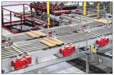
**Inverter-only mode (S9)**Motors operating on the inverter only, with movements at different speeds, for transporting, accelerating, and decelerating
