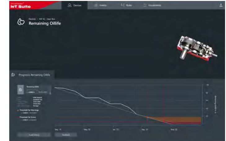
DriveRadar® IoT Suite: Prediction of the remaining oil service life and oil change
