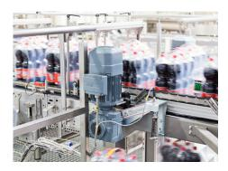
Asynchronous motors in IE3
