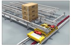
Pallet transfer shuttlesConveying systems in logistics centers
