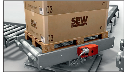
Materials handling technology with changes of direction Turntable, trolley
