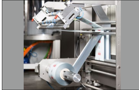
Machine with web material running through it and with winding units and tension shafts
